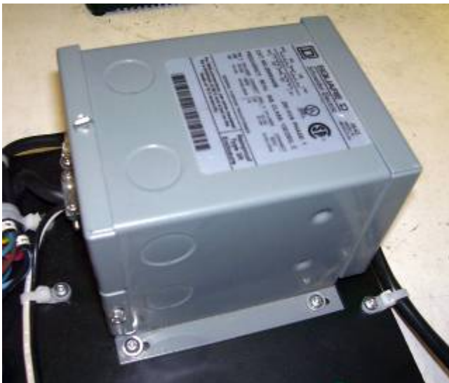
Transformer ASSY .25KVA Square D PK/TR (Part # EX023175)
